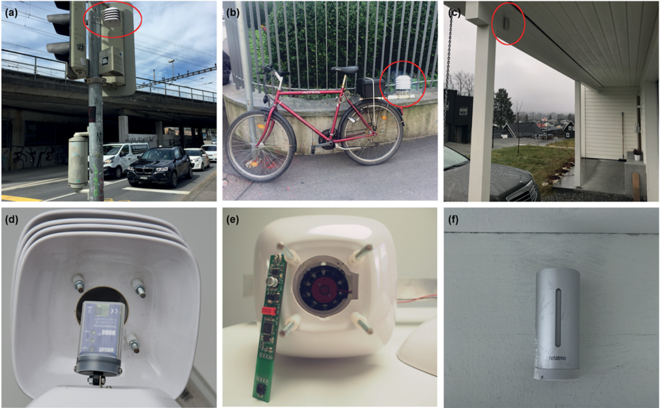
Figure 3: Illustration of the measurement set up (top row) and the measurement devices (bottom row) for the LCD (a & d), the BCY (b & e), and the CWS (c & f). Red ellipses highlight the location of the measurement device (Photo credits: M. BURGER (a), M. GUBLER (b), E. LUNDSTAD (c) and (f), P. DUSCHLETTA (d), L. MEYER (e)).
