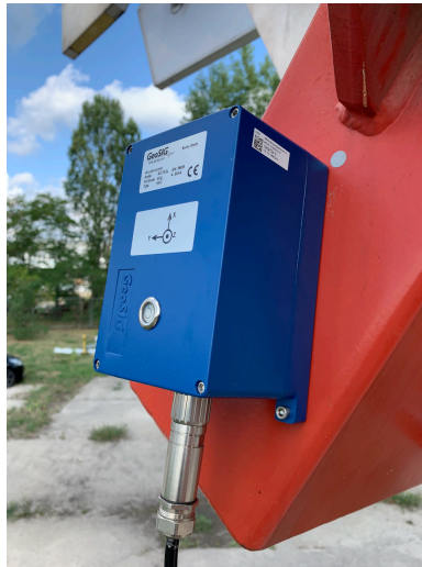
Figure 5.5.: One of the three GeoSIG [166] sensors attached to the MST prototype (Berlin, 2019).
