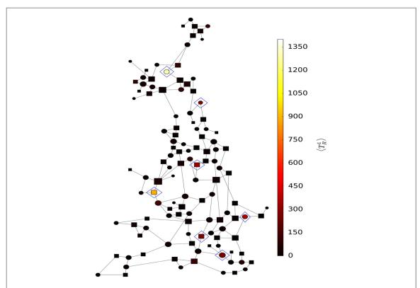
**Figure 5.** Network topology of the power transmission grid of the United Kingdom (comprising N=120 nodes) with second-order Kuramoto-type nodal dynamics. Circular nodes denote net generators while square nodes are net consumers. The size of each symbol is proportional to the degree, and its colour corresponds to the  $\langle T_R^1 \rangle$  value of the respective node. The seven nodes further encircled by blue diamonds comprise the *slow* nodes of the grid in our simplified model.
