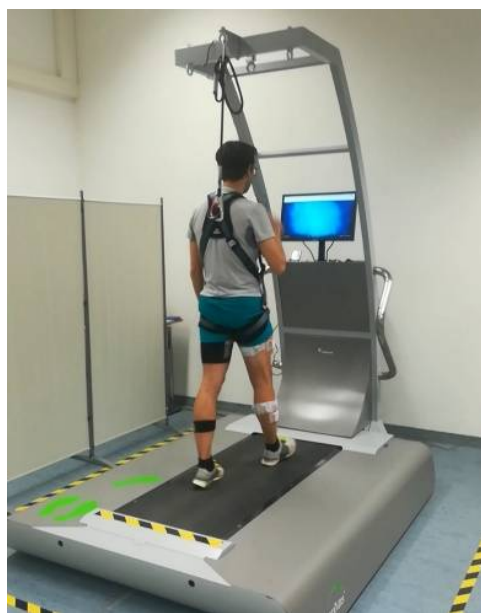
Figure 1. Example of a participant placed on the treadmill with the harness worn and the sensors positioned on the body segments of interest. The sensor on the pelvis was placed under the t-shirt.
