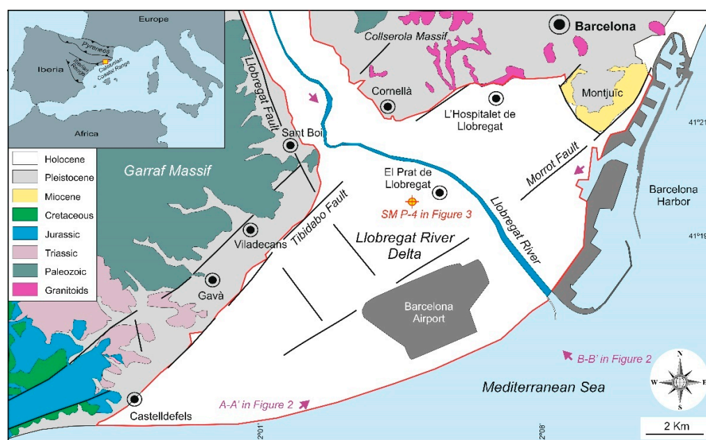
Figure 1. Geological sketch map of the LRD area (red line contour), modified and updated from Medialdea and Solé-Sabarís [4,5], Alonso et al. [6], and Gámez et al. [7]. Geological cross-sections A-A' and B-B' are displayed in Figure 2. Geotechnical borehole SM P-4 with granulometry data are displayed in Figure 3.
