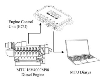
Figure 4 Engine fault tracking system
