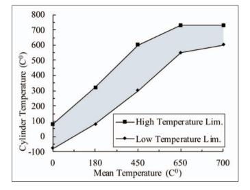
Figure 2 Change of cylinder temperature alarm limits depending on average temperature for each cylinder
