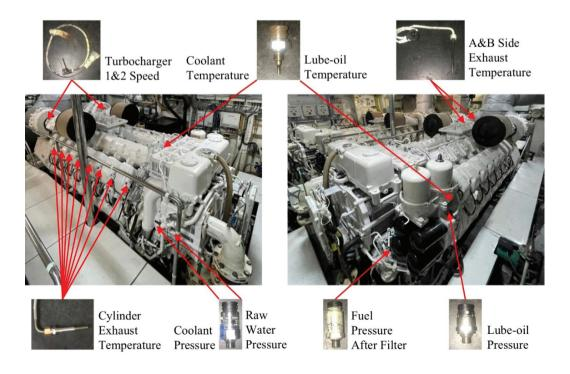
Figure 3 Locations of sensors on four-stroke marine diesel engine
