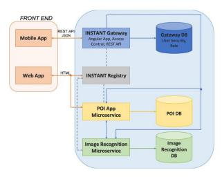
Fig. 1. Block diagram of the INSTANT system architecture.
