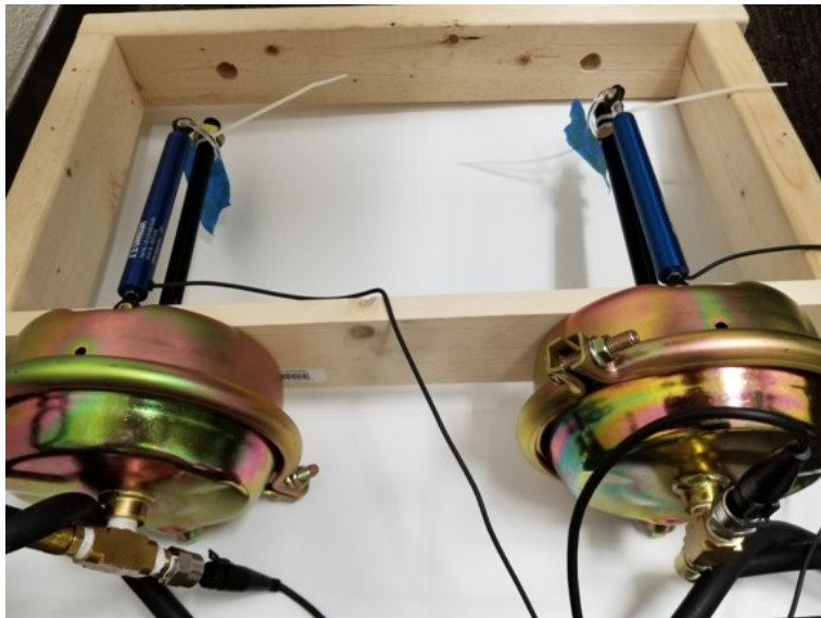
Figure 3.1: Wooden Frames and Rear Brake Setup
