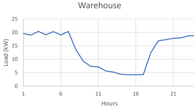
Figure 6: Load Profiles of the Representative Loads on the first 24 hours of the year.
