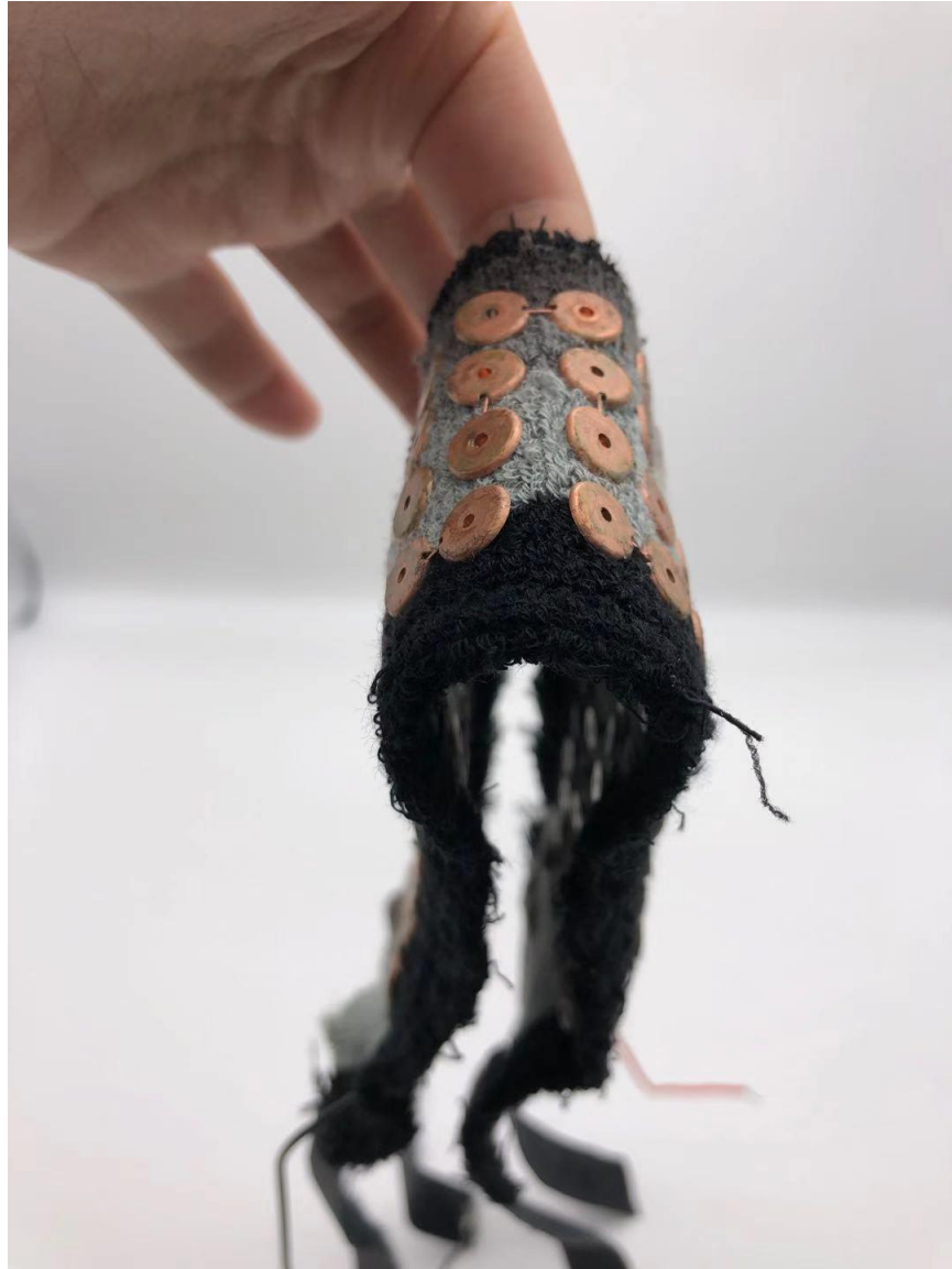
Figure S3. Demonstration of the f -TEG headband's flexibility.
