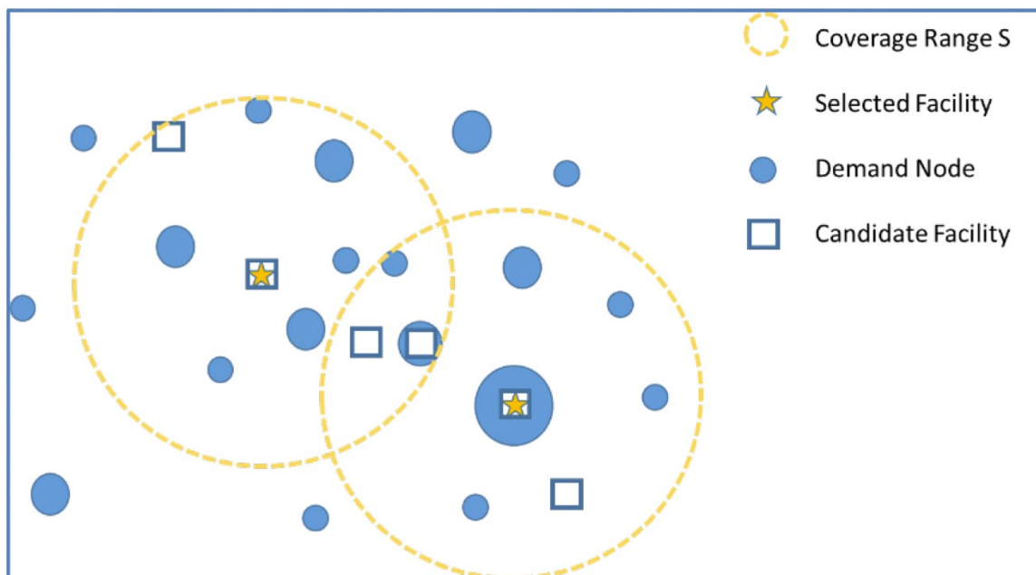
Figure 4-1. An illustration of locating facilities with the maximal covering location problem (MCLP), with demand nodes sized proportional to the amount of notional demand.
