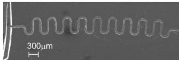
Figure 54: Micro-Snake NiTi Actuator Machined Using Laser from a 120µm NiTi Sheet (Reprinted from [41])
