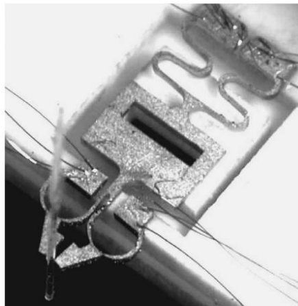
Figure 56: A Micro-Gripper Laser Machined out of SMA Sheet (Reprinted from [46])
