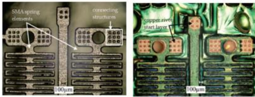
Figure 58: Galvanic Riveting of Micro SMA Springs (Reprinted from [44])
