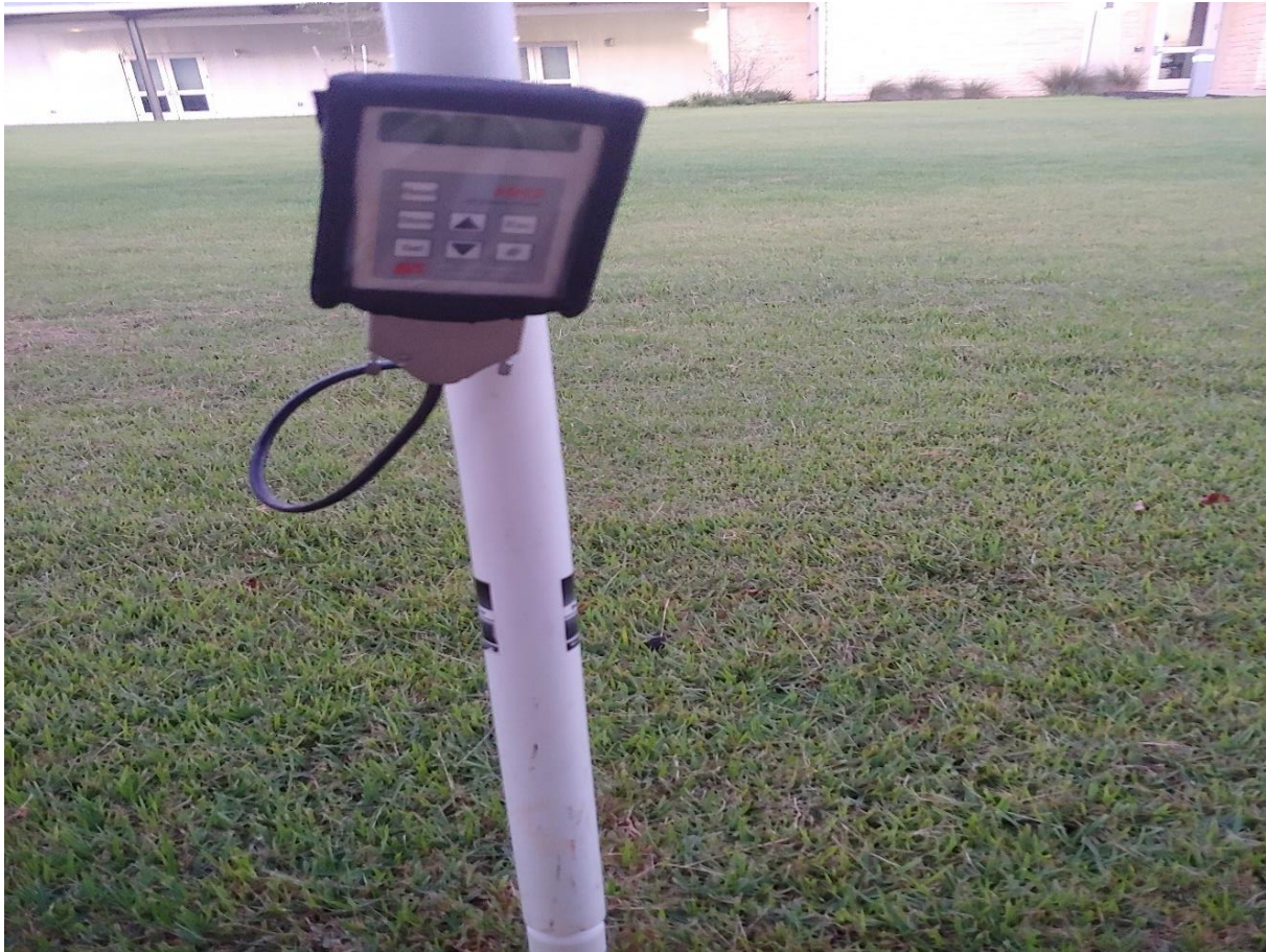
Figure 3.2: Dynamax TH_2O moisture meter used for measuring soil moisture content
