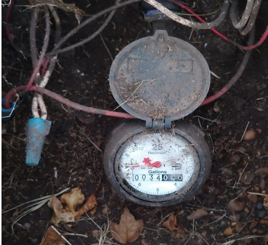
Figure 3.4: Flowmeter used in TAMU Turfgrass Laboratory for measuring applied irrigation volume
