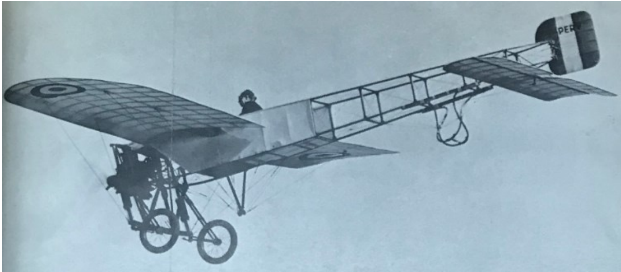
Figure 2.4. The Blériot XI, an iconic airplane of the earliest era of heavier-than-air flight, was the most widely used monoplane. “Blériot XI,” box 5, folder 5, COR, BNA.
