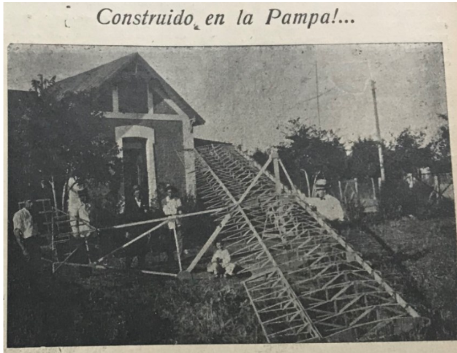
Figure 4.15. Caption reads: “This glider is currently under construction in Santa Rosa, La Pampa, by various aficionados from that town, according to the plans published in this magazine.” It is unclear if it ever flew. Ciencia Popular , January 1931, 580.
