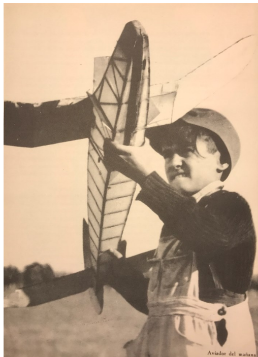
Figure 7.11. The “Aviator of tomorrow”. The wooden internal structure of the model, wrapped in paper, are evident here. From a promotional book published by the Secretaría de Aeronáutica. S.d. Aeronáutica, La Aeronáutica nacional , 137.
