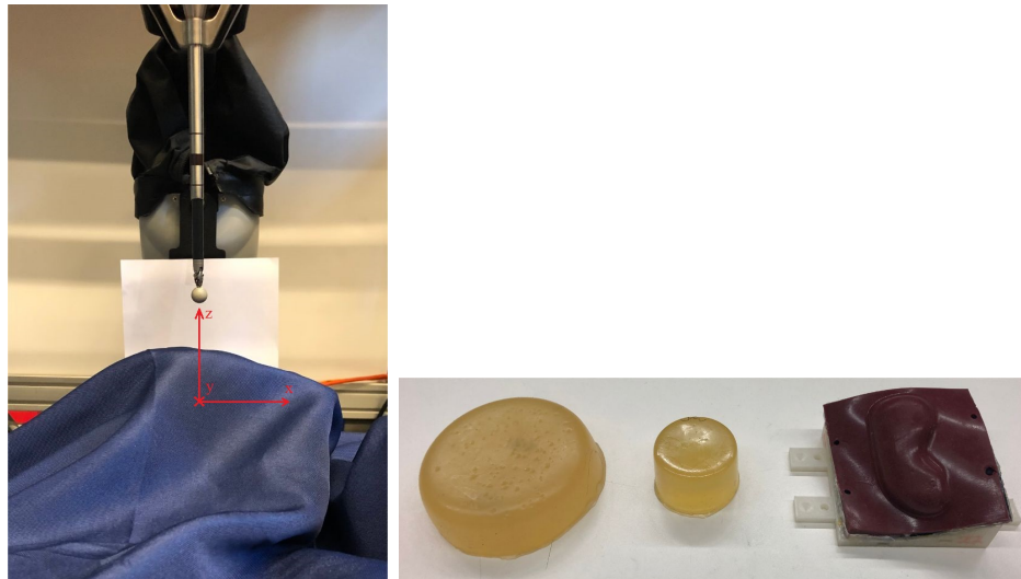
Figure 2-8. dVRK test bench horizontal configuration for pilot study. A small round marker is attached to the tip to prevent damage to soft phantoms. Also depicted are the phantoms used in the pilot study, with increasing order of stiffness from left to right. They are set to equal height and covered with a drape during the pilot study.
