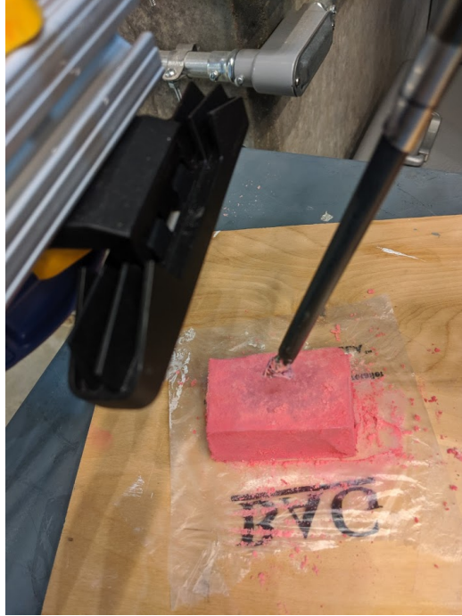
Figure 4-1. Deformable phantom setup. The RGBD camera is mounted above the workspace on the left. The phantom is coated with spray paint and potato starch to improve its visibility to the depth camera.
