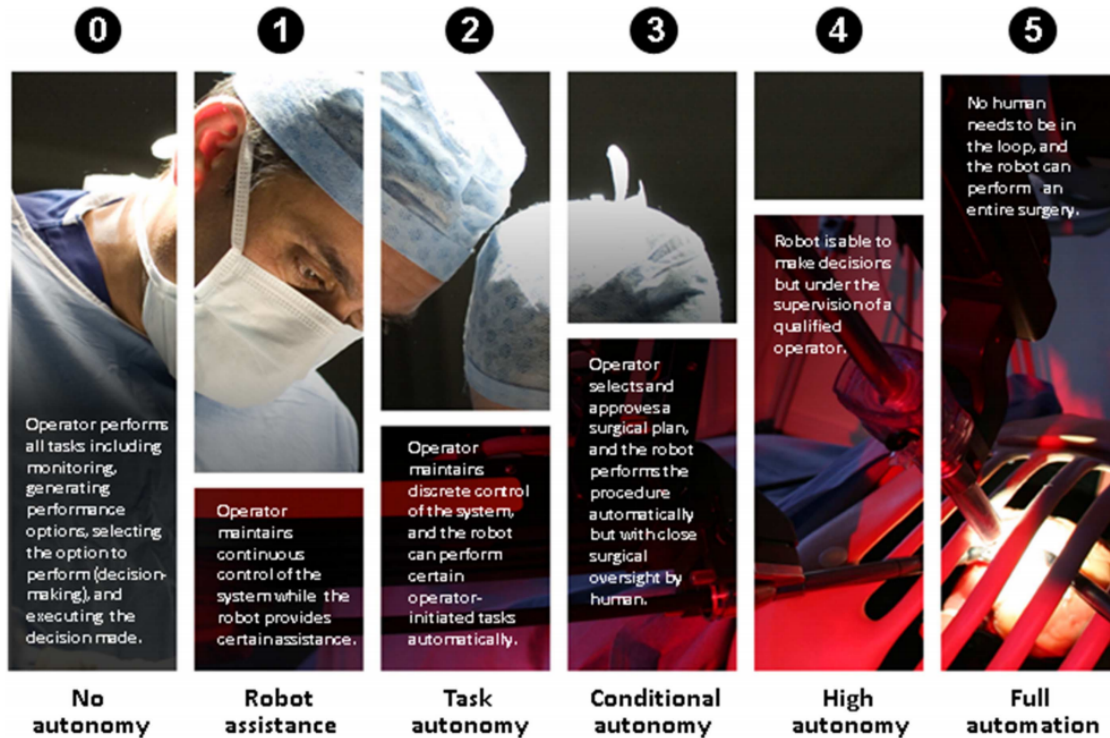
Figure 1-2. Proposed levels of autonomy [13]. Currently, teleoperation systems for soft-tissue procedures are at level 0 or 1. Robots operating at up to level 3 have been used in other fields such as orthopedics and ophthalmology, where the environment is better defined.
