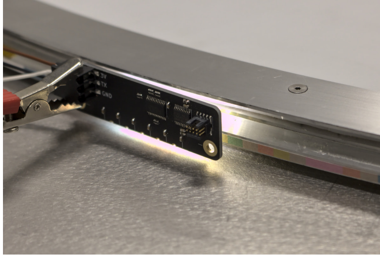
Figure 6.5: The fully assembled encoder prototype is shown installed in a position to read an encoder track installed on the edge of a \sim 1.5 m diameter ring.
