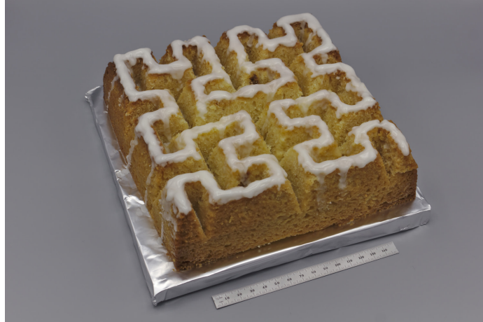
Figure 4.6: An alternative realization of the absorber geometry is shown. Due to the geometry's size, it will likely not perform well at millimeter wavelengths. While the material's dielectric properties have not been measured, the imaginary component is likely too low for good electromagnetic performance; it is edible, however.
