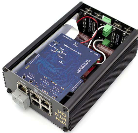
Figure 3.7: The assembled VPM control electronics are shown. Besides the logic board and the voice-coil-driver board, additional PCBs are used to hold connectors, route electrical signals, provide mechanical support, and serve as faceplates. This allows for the electronics to be assembled into a compact extruded-aluminum enclosure.
