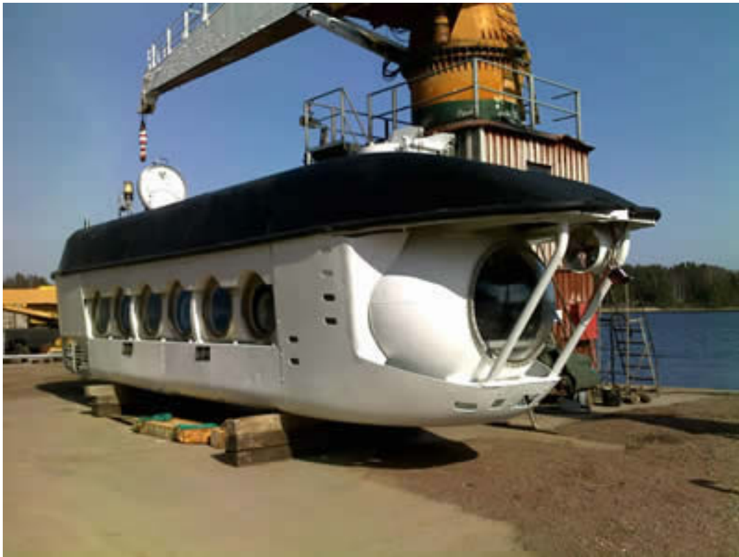
Figure 2-4 A typical tourist submersible (T-SUB) [68]
