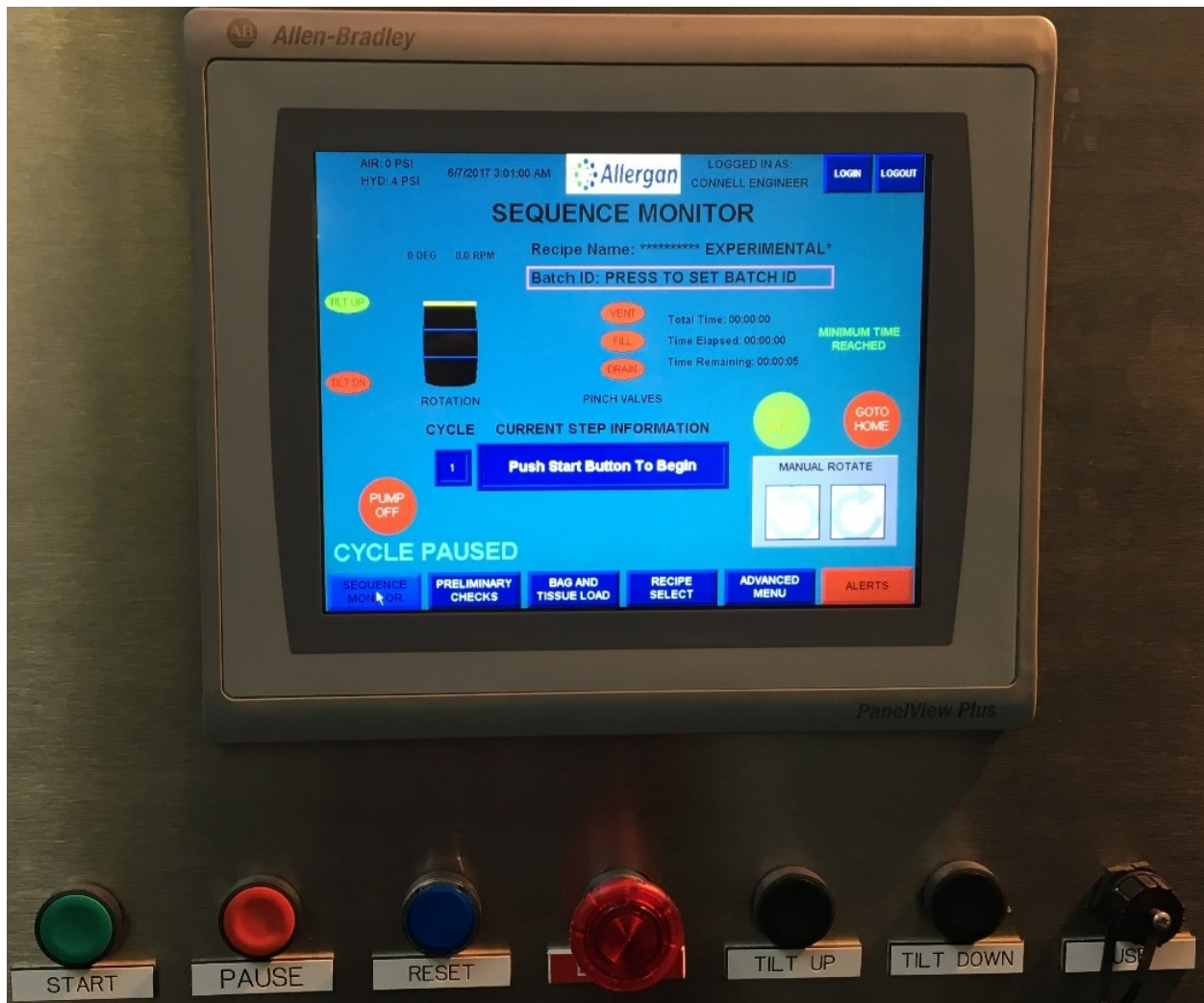
Figure 1-2 An Allen Bradley Touchscreen HMI [10]
