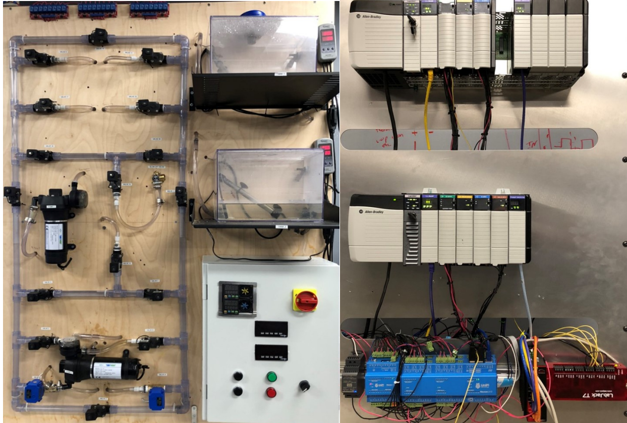
Figure 3-6 The Water Chilling System with Sensors, Actuators (left), and Controllers (right)
