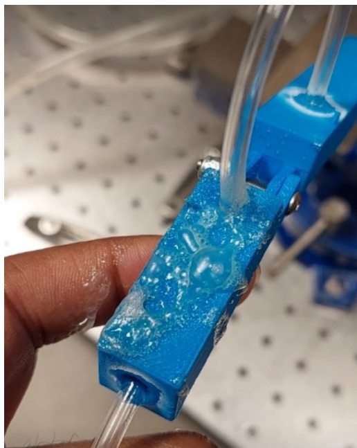
Figure 10: Pressure testing, leaks detected.
