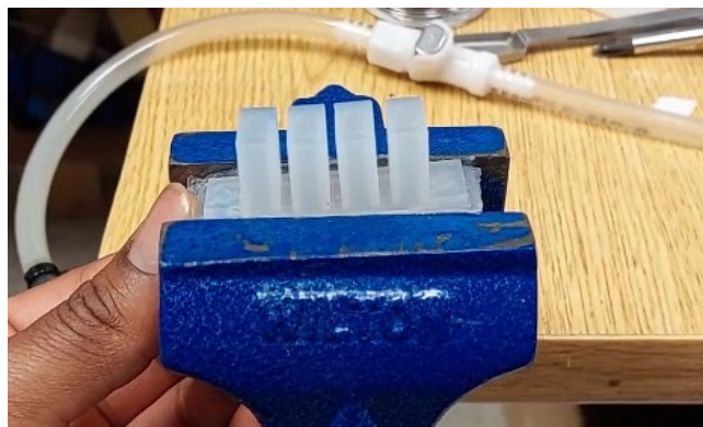
Figure 16: Pressure test set up for the soft actuator
