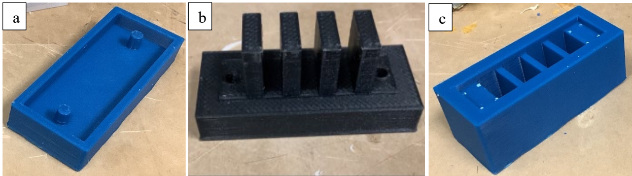
Figure 13: Bellow molding components (a)Lower base plate (b) Upper inner form (c) Upper outer form
