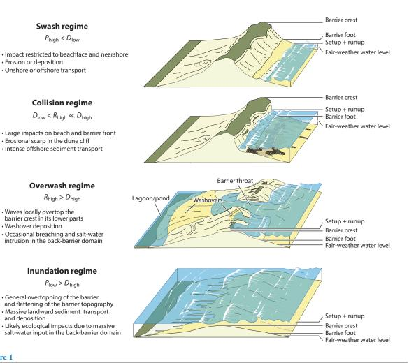
The Sallenger (2000) storm-impact scale.  $D_{high}$  denotes the height of the barrier crest,  $D_{low}$  denotes the height of the barrier foot,  $R_{high}$  denotes the highest action of the waves (tide + surge + setup + runup), and  $R_{low}$  denotes the lowest action of the waves (tide + surge + setup). Figure adapted with permission from Goslin & Clemmensen (2017); copyright 2017 Elsevier.
