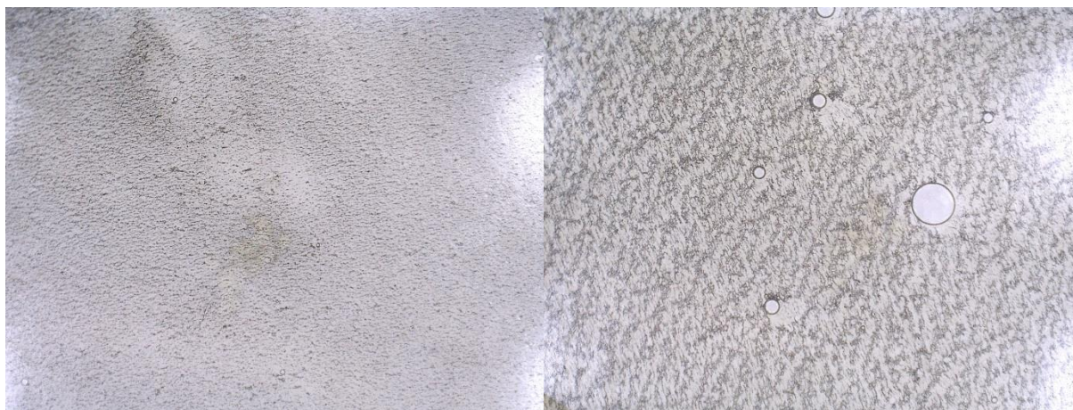
Figure 1. Micrograph of a ferromagnetic liquid in a uniform magnetic field (left), with multiple changes in the orientation of the magnetic field (right).
