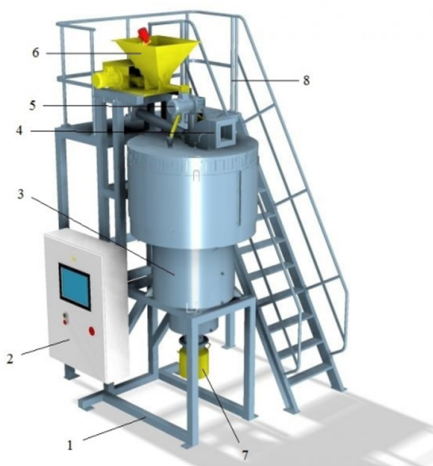
Figure 2. Experimental-industrial centrifugal reactor “TSEFLAR™” of the drum type: 1—frame; 2—control board; 3—cooler; 4—air duct; 5—drum drive; 6—tank for raw material; 7—tank for the thermally treated product; 8—processing area.
