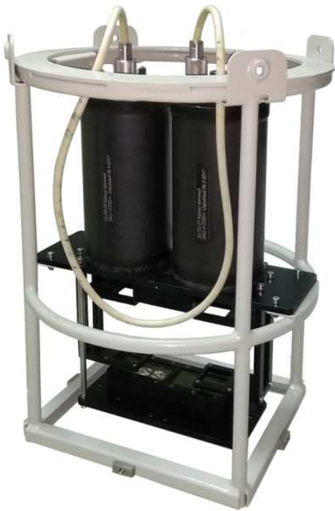
Fig.2. Digital holographic camera (DHC)
