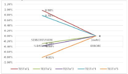
Graph.3: Error percentage for tests calculated with sensor fusion
