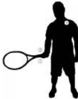
Fig. 1; Example of sensors positioning, 1 Racket, 2 Wristband 3 Chest.
