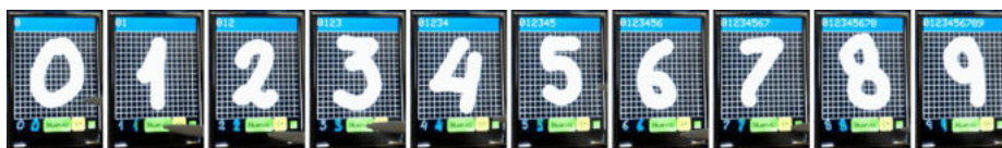
Fig. 4: ATmega2560 example integrating model, inference functions, graphics and touchscreen functions in 24Kib of program memory and 6Kib of RAM.
