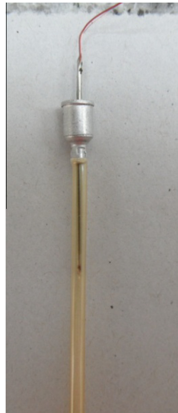
Fig. 1. Straw initially filled with pure water with the thermocouple threaded into the needle and mounted into the straw to avoid radial movement during the experiment.
