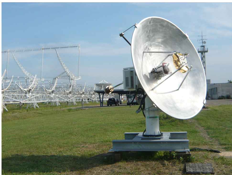
Fig. 14 Broadband 2.4 m antenna MBL1 installed at the campus of Medicina Radio Astronomical Station of INAF in 2018
