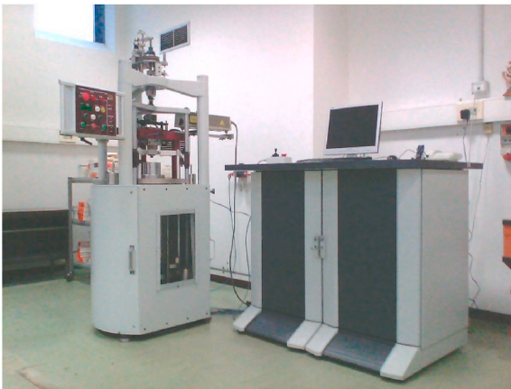
Fig. 2. INRiM's Rockwell preliminary hardness standard machine.
