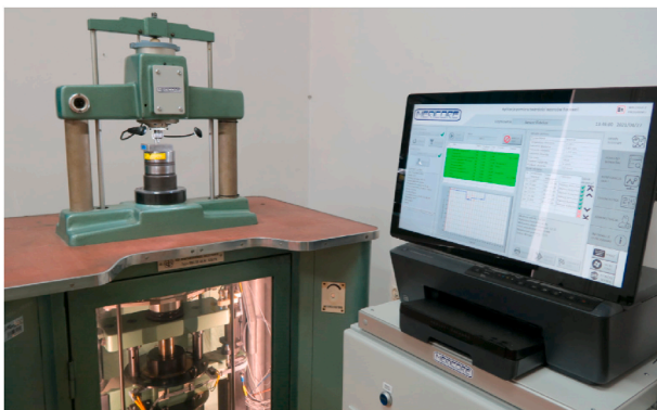
Fig. 3. GUM's Rockwell hardness standard machine (HSM-S02) equipped with the Renishaw RESOLUTE system, which consists of an optical encoder (head) and a stainless steel belt scale with laser-engraved absolute code and a computer with dedicated software (control and device diagnostics application written in LabVIEW) for data analysis and archiving.
