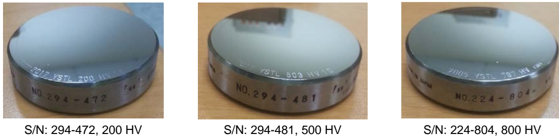
Figure 3. Transfer Standards for HV1 and HV30 Scales.
