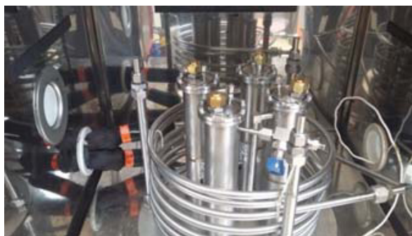
Fig. 8. Measurement chamber of the CETIAT humidity generator.
