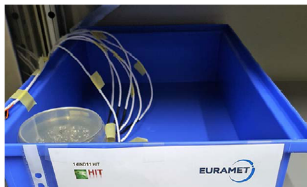
Fig. 16. A photograph showing a measurement setup for measuring small gradients of temperature and humidity in a Petri dish stack.
