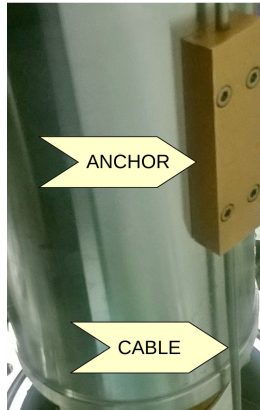
Figure 2: Copper block for thermal anchoring the coaxial cable to the cylindrical first stage shield of the cryocooler
