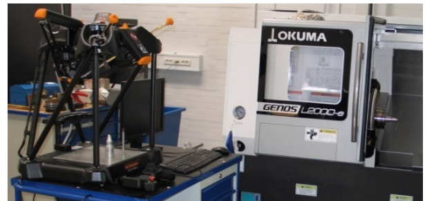
Figure 40. Master for process control in the production using a CNC gauge by Renishaw (source: DTU).
