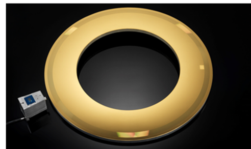
Figure 33. Angular grating with 400 mm diameter consisting of 2^{17} = 131\,072 graduation lines resulting in angular intervals between adjacent lines of 9.89 arcsec and one reading head being the core components of an angular encoder (source: EURAMET).
