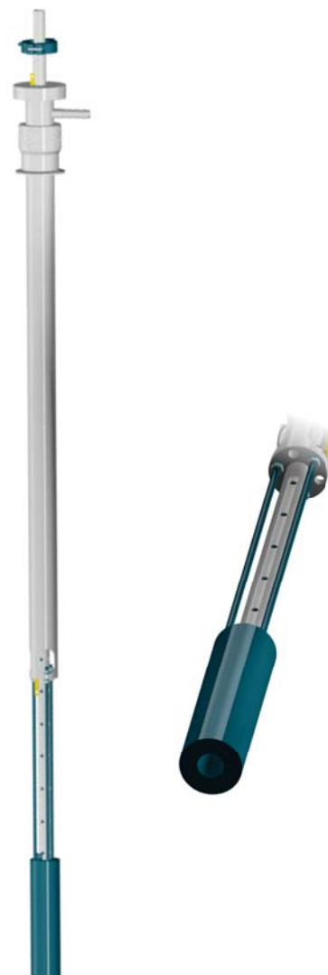
Fig. 1. A computer rendering of the cryomagnetic probe assembly: (left) side view; (right) front view, showing the magnet bore.
