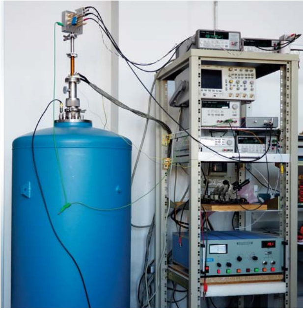
Fig. 7. Overall view of the measurement setup for DC characterisation. On the left, the liquid helium dewar, with the coaxial probe inserted. On the right, the rack of electronic instrumentation.
