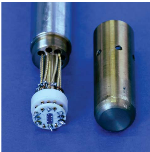
Fig. 3. The bottom side of the insert, which slides into the cryomagnet bore. The brass shield (right) has been removed, to show the TO-8 socket, which hosts a GaAs device on its TO-8 holder, and the 9 coaxial electrical lines.
