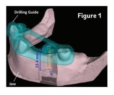
**Figure. 1:** Trial of a dental drilling guide produced by additive manufacturing for the drilling of holes to fit dental implants into artificial jaw models with only few abutment teeth. The drilling angle  $\alpha$  and the drilling depth were measured by means of computed tomography. Source: PTB
