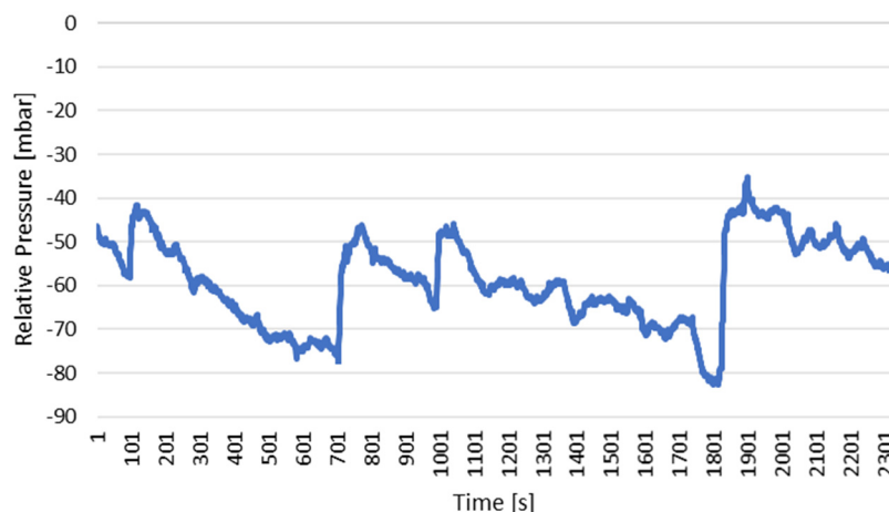
Figure 10. Pressure in the bottom zone of the gasifier fueled with briquettes (30% weight) and woodchips (70% weight).
