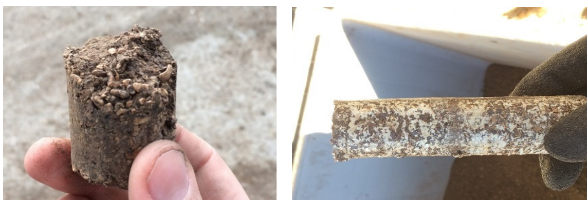
Figure 6. Briquette of olive pomace (left) and briquette of mix olive pomace (80% w/w) and sawdust (20% w/w) (right).
