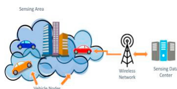
Fig. 2. Architecture of vehicular mobile crowdsensing systems
