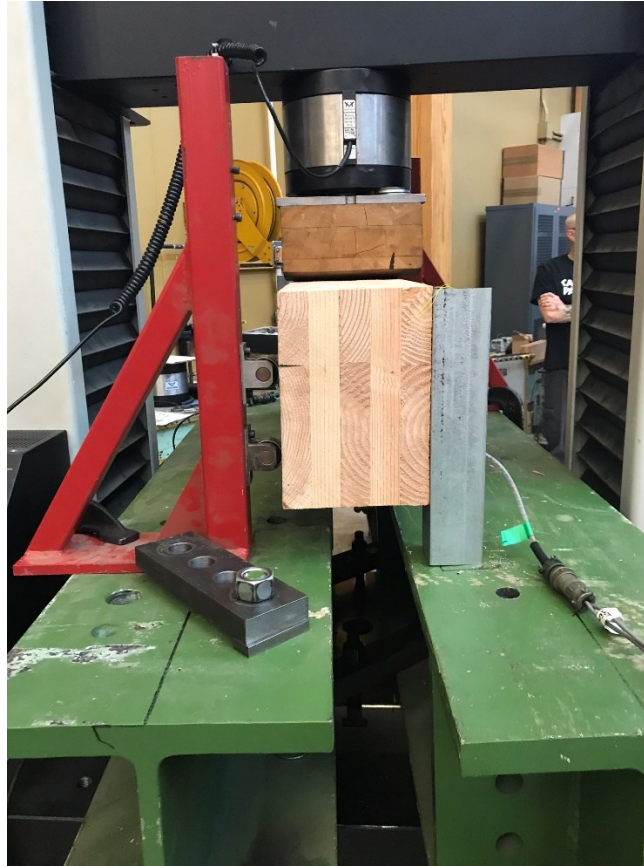
Figure 2.9 End view of test set up showing that samples were kept in plane during loading.
