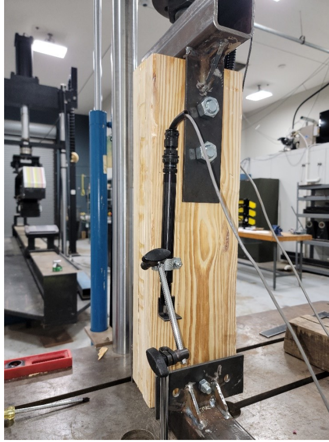
Figure 3.2 Test set up with LVDT attached to monitor movement of fastener.
