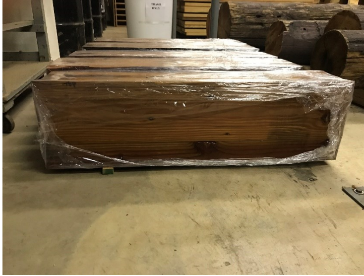
Figure 2.4 Samples end grain wrapped in plastic to limit moisture movement and imitate conditions of whole wall more closely.
