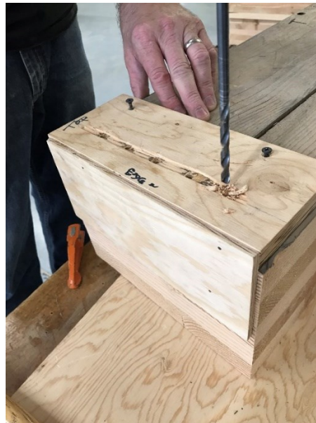
Figure 2.3 Jig utilized for uniform predrilling of CLT specimens.
