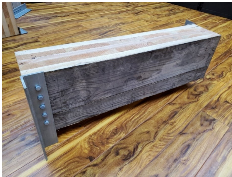
Figure 2.1 Typical example of 5-Ply CLT sample
