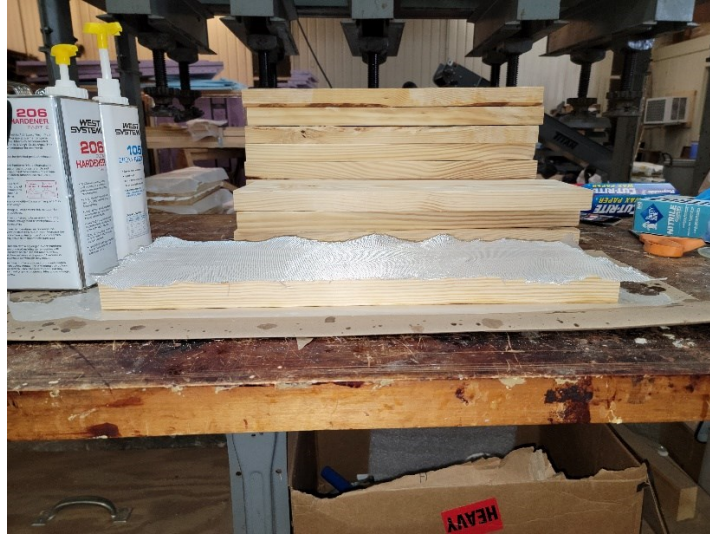
Figure 3.1 Assembly of samples, laying fiberglass on wood and epoxy application.
