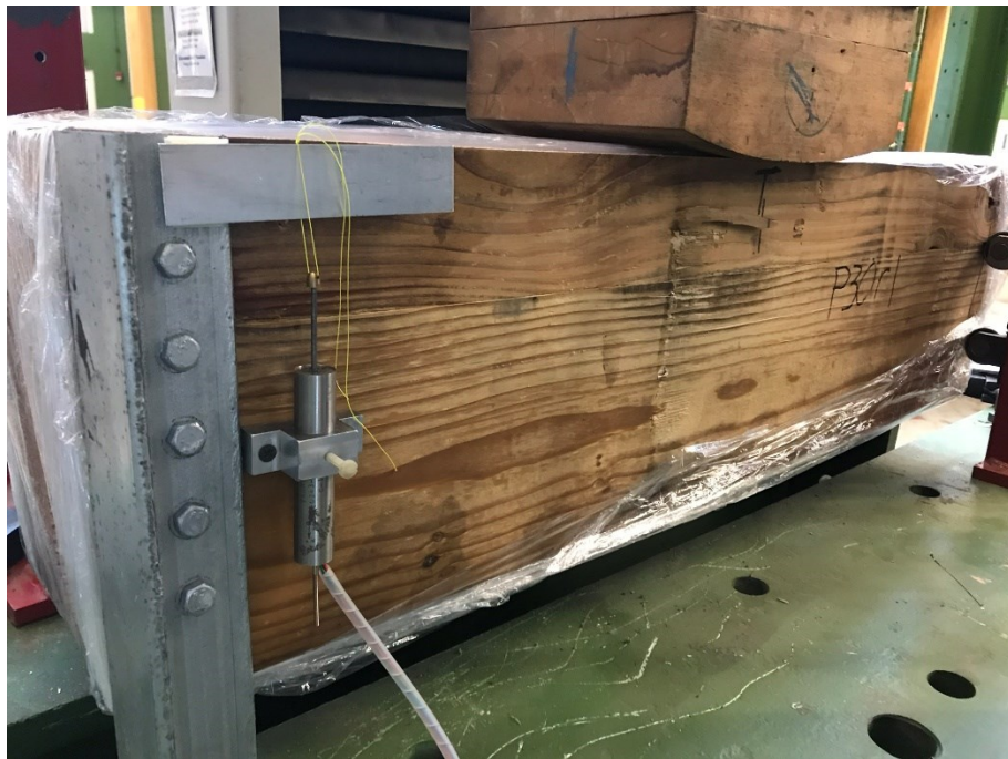
Figure 2.8 LVDT utilized to track movement of bolts under loading.
