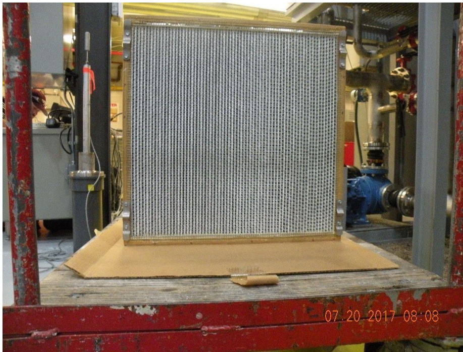
Figure 2.3 Pre-Filter Loading Test
