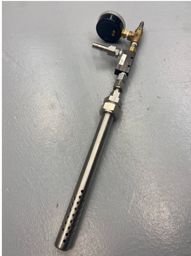
Figure 3.12 Injection Manifold Assembly.
