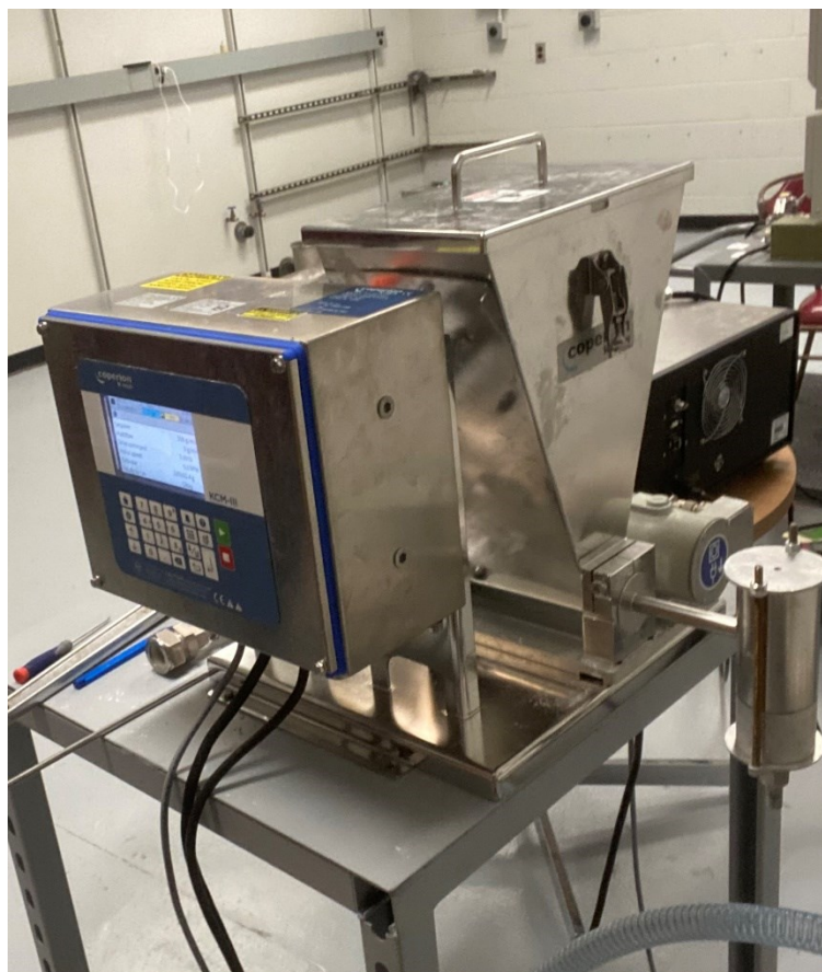
Figure 3.27 Powder Feeder for \text{Al}(\text{OH})_3 and ARD.
