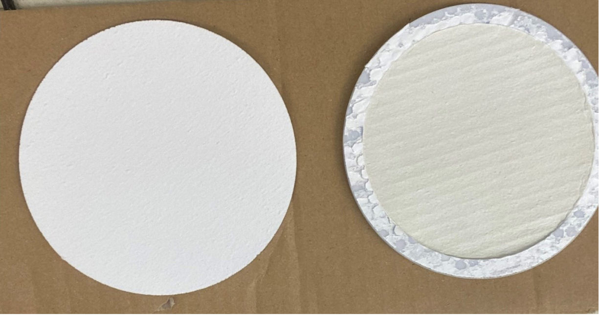
Figure 4.4 New vs Baked Filter Coupon
