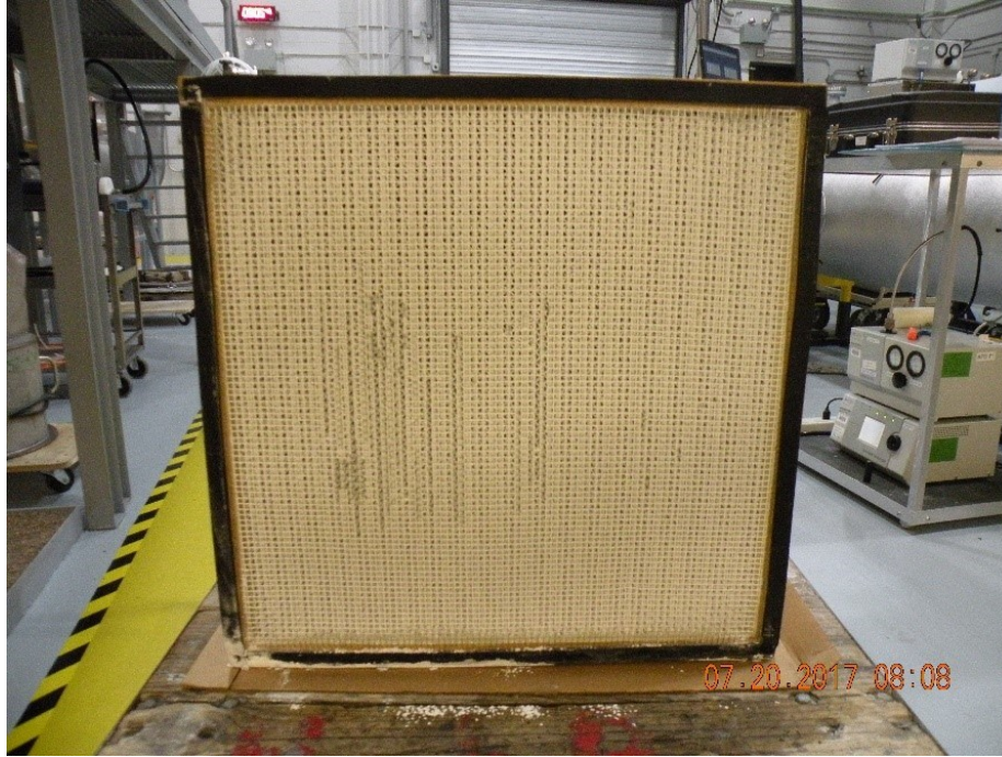
Figure 2.4 Post-Filter Loading Test
