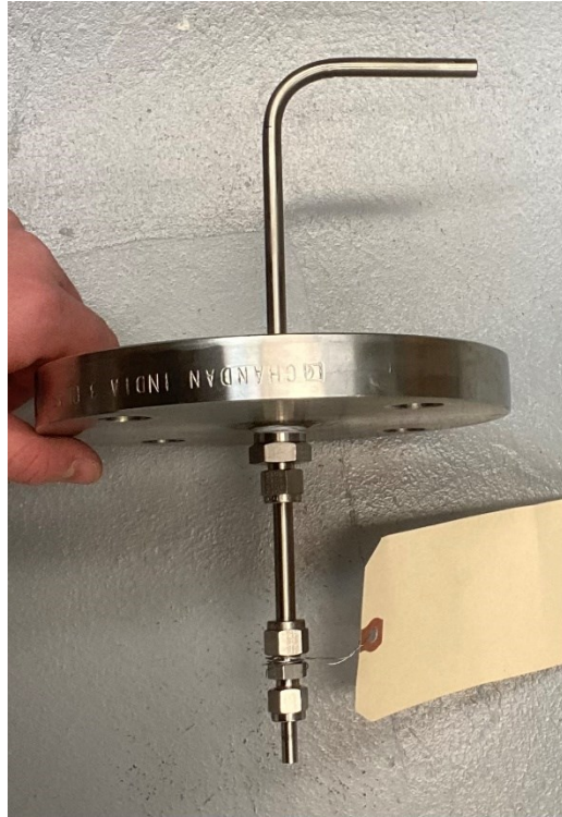
Figure 4.10 0.27-inch ID Sampling Probe
