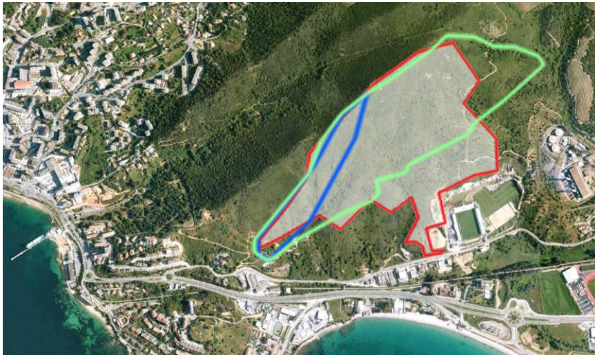
Fig. 9. Simulations results and observations for the Vazzio fire. Blue: simulated fire contour at 15:30 (after 1h), Green: simulated contour at 18:30, Red: final observed contour of the fire.
