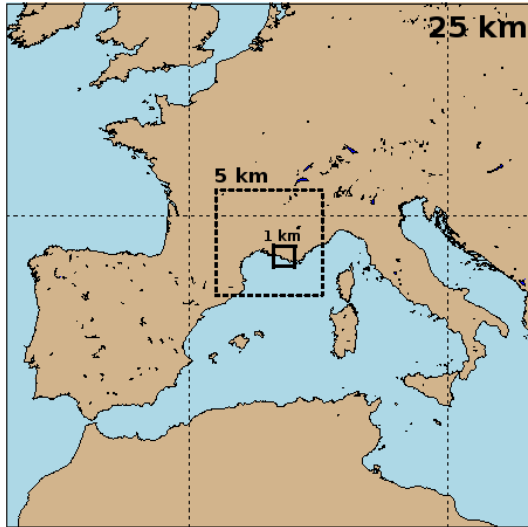
Figure 1: Meso-NH nested domains used in the Lançon-de-Provence case study from the coarse 25-km grid down to the fine 1-km grid.
