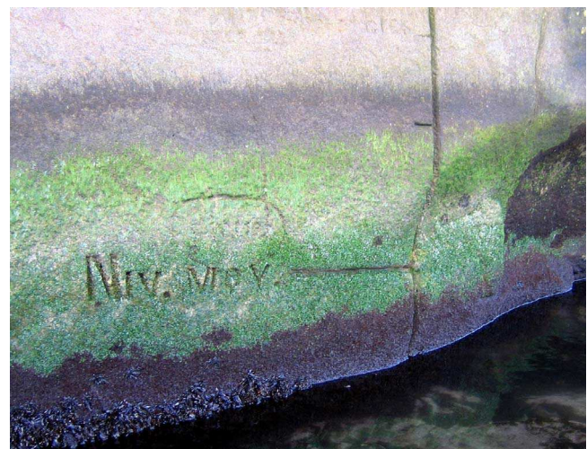
Figure 2. Photograph of the engraved mark of 1874 at Saint Paul Island with the inscription “Niv. moy.” (“Mean level”). The horizontal line is 1.9 cm wide in width at the intersection with the vertical line (photograph taken in 2009).
