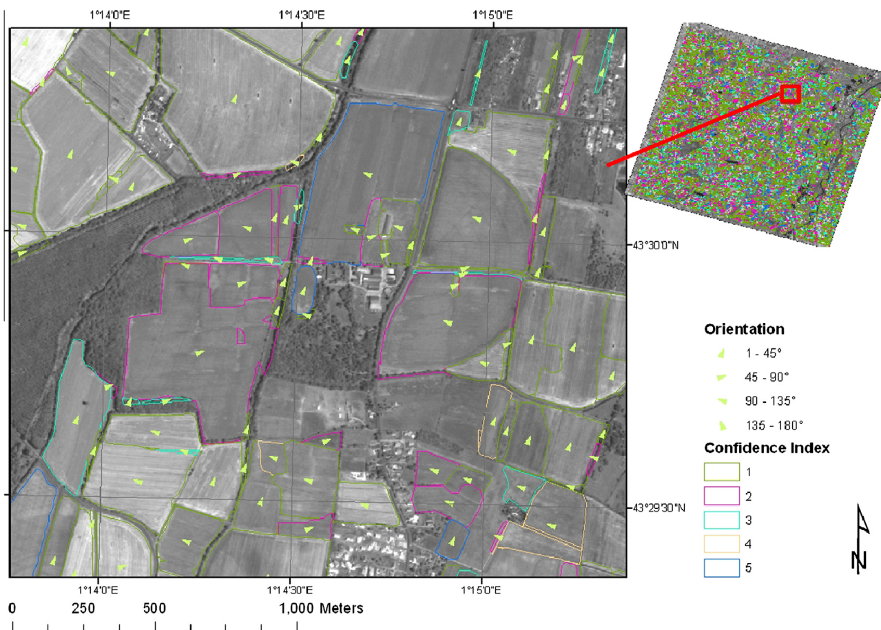
Fig. 19. Row orientation map produced using a multi-temporal approach. Each plot is associated with a confidence index ranging between 1 (high confidence) and 5 (low confidence).
