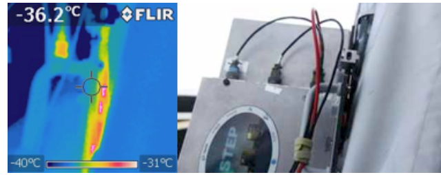
Fig. 15 Photographs of the ASTEP camera box at the interface with the telescope. Left: IR photograph showing the warm plume at the interface between the camera box and the telescope tube. Right: Visible photograph of the camera box and telescope tube.
