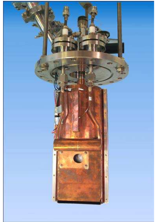
Figure 3 Overall view of the device with 80 K shield
