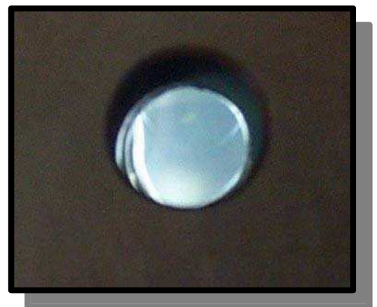
Figure 4 Hydrogen target : solid growth
