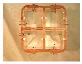
**Fig. 16.** Top view of the detector tower of the CUORICINO experiment. Each plane of the tower comprises four detectors, weighing 760 g each, except for two of the lower planes, each comprising  $9 \times 340$ g. The energy of an interaction is measured by the impedance variation of a Neutron Transmuted Doped (NTD) Ge sensor. These detectors are operated at a temperature of  $\sim 10$  mK in the Gran Sasso underground laboratory (Italy)
