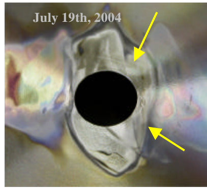
Sputtering impacts on the first electrode of the accelerating tube.
