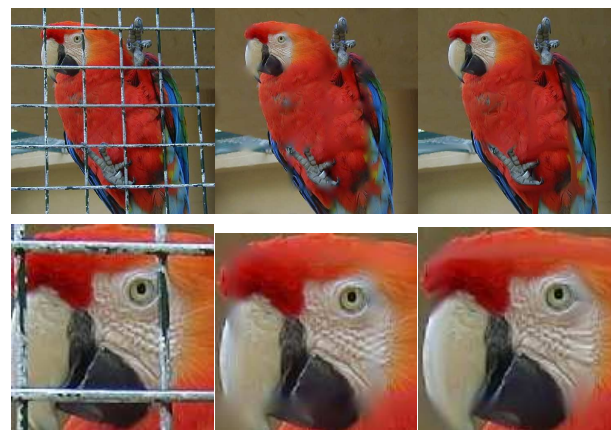
Fig. 3. Original (left), ECM inpainting (middle) and PDE inpainting (right).
