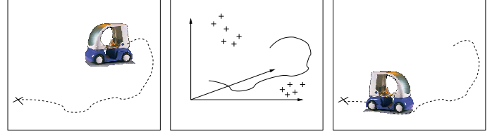
Fig. 4. Principle of vision based localization. 1) vehicle freely moves and records a video sequence. 2) trajectory and visual features of the video are reconstructed. 3) vehicle can localize itself and take the same path.
