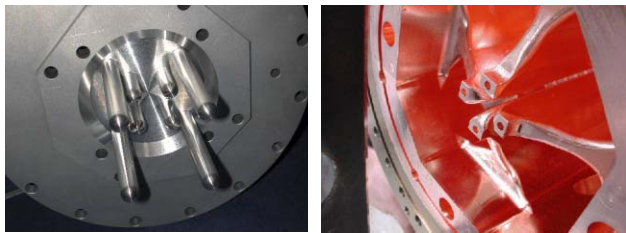
Figure 3: End plate with DR and QR, and vane ends.
